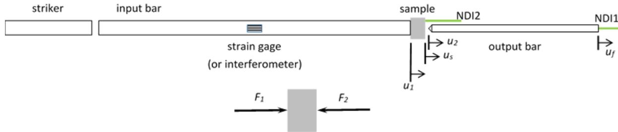
Multiple tests can be conducted on a single sample if:
